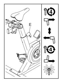
saddle post upward or downward, release the adjustment handle into an adjustment hole in the saddle post, and firmly tighten the adjustment handle four turns. Make sure that the adjustment handle is engaged in an adjustment hole. Then, pull the adjustment handle outward, turn it so that it points downward as shown, and then release it.
