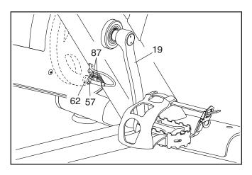
Next, turn the Left Crank Arm (19) until a Magnet (62) is aligned with the Reed Switch (57). Slide the Reed Switch slightly toward or away from the Magnet. Then, retighten the M4 x 20mm Screws (87).
