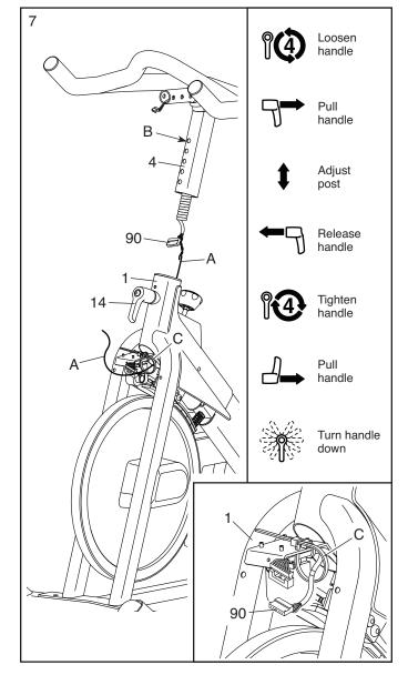
8. See the inset drawing. Connect the connector on the Handlebar Wire (90) to the connector on the Frame Wire (82). Tip: The wire connectors should slide together easily and snap into place with an audible click. If they do not, turn one connector and try again.
