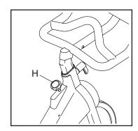
IMPORTANT: When the exercise bike is not in use, tighten the brake knob (H) completely.
