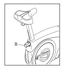
the knob is engaged in one of the adjustment holes in the seat post. Then, turn the knob clockwise to tighten it.
