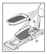
To lower the ramp, press the latch button (G), pull the ramp handle (H), and lower the ramp to the desired incline level. Then, release the latch button and engage the latch pin into one of the adjustment holes in the frame. Make sure that the latch pin is firmly engaged in one of the adjustment holes in the frame.
