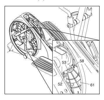
Next, rotate the Pulley (61) until a Magnet (58) is aligned with the Reed Switch (53). Slide the Reed Switch slightly toward or away from the Magnet. Then, retighten the M4 x 16mm Screw (52). Rotate the Pulley for a moment.
