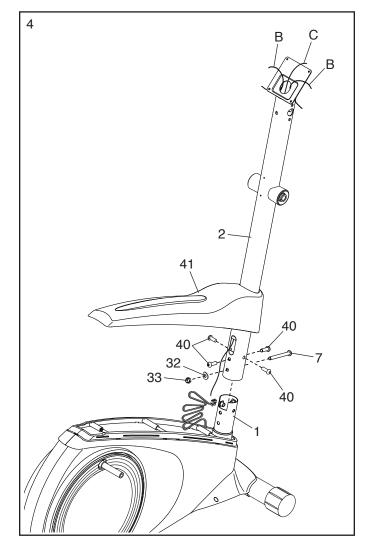
See the inset drawing. Locate the wire tie (C) in the lower end of the Upright (2). Tie the wire tie to the Wire Harness (73). Next, pull the upper end of the wire tie until the Wire Harness is routed through the Upright.
