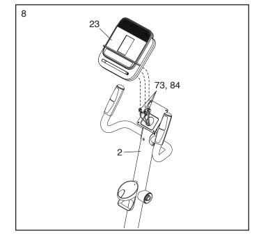
9. Insert the excess wire into the Upright (2) or into the Console (23).
