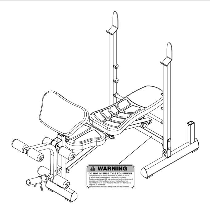
The warning label shown here has been placed on the Cross Brace. If the label is missing or illegible, please contact Customer Solutions via email: service@puretecfitness.com for replacements. Apply the label in the location shown.
