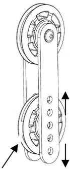
Adjust the tension of the Cable System by moving the position of lower Pulley on the Double Floating Pulley Brackets.
