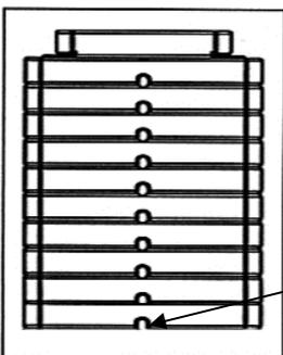
Slide weight plates onto Guide Rod from top to bottom.
