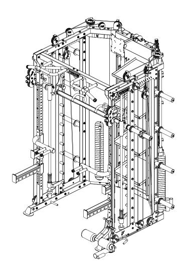
2 Connect link frame-90, selector frame-91, TV bracket-93 use  $\Phi$ 10x85xM10 shaft-92,  $\Phi$ 10 washer-7, M10 lock nut-6 Attach them to the mainframe use M10x20 hexagon bolt-94,  $\Phi$ 10 washer-7,  $\Phi$ 10 spring washer-14
