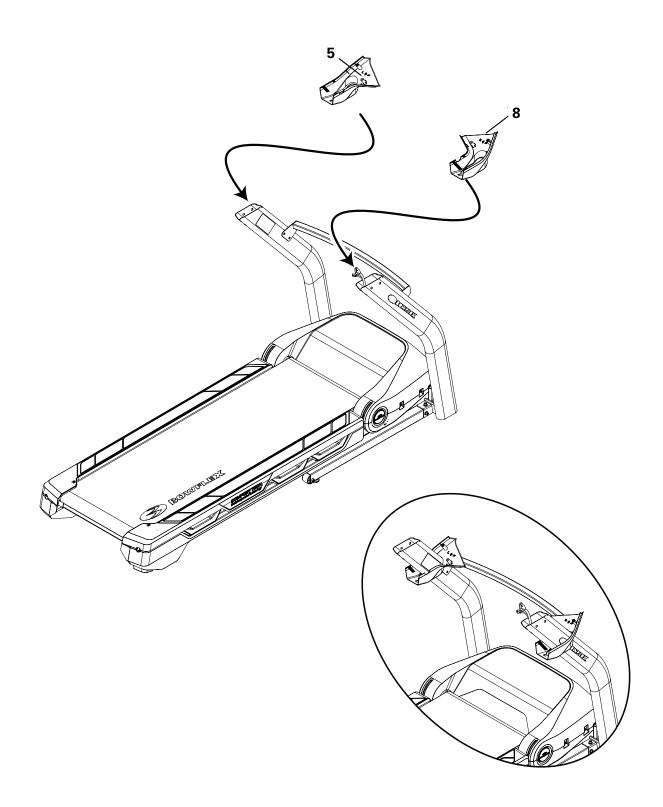
4. Connect the Cables and Attach the Lower Junction Covers and Console Assembly
