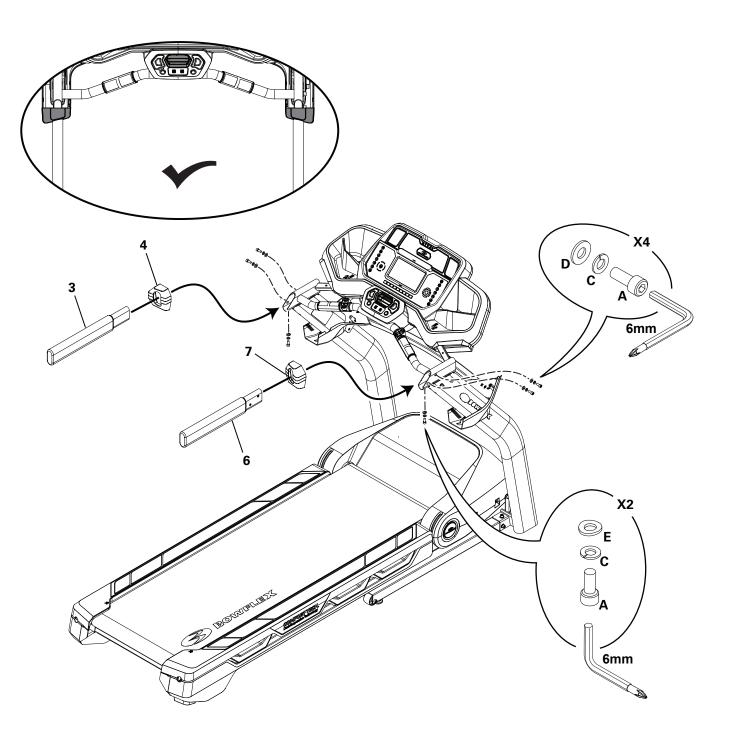
7. Snap the Upper and Lower Junction Covers into Place and Secure with Hardware to the Frame Assembly
