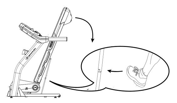
4. The hydraulic lift is set up to drop lightly. Hold onto the walking deck until approximately 2/3 of the movement down. Make sure that you use proper lifting technique; bend your knees and keep your back straight. Lower the weight with your legs. The walking deck can possibly drop quickly in the last part of the movement.
