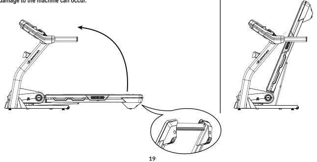
7. Make sure that the locking mechanism is engaged. Carefully pull back on the walking deck and make sure that it does not move. When you do this, keep clear of movement path in case the treadmill lock is not engaged.
